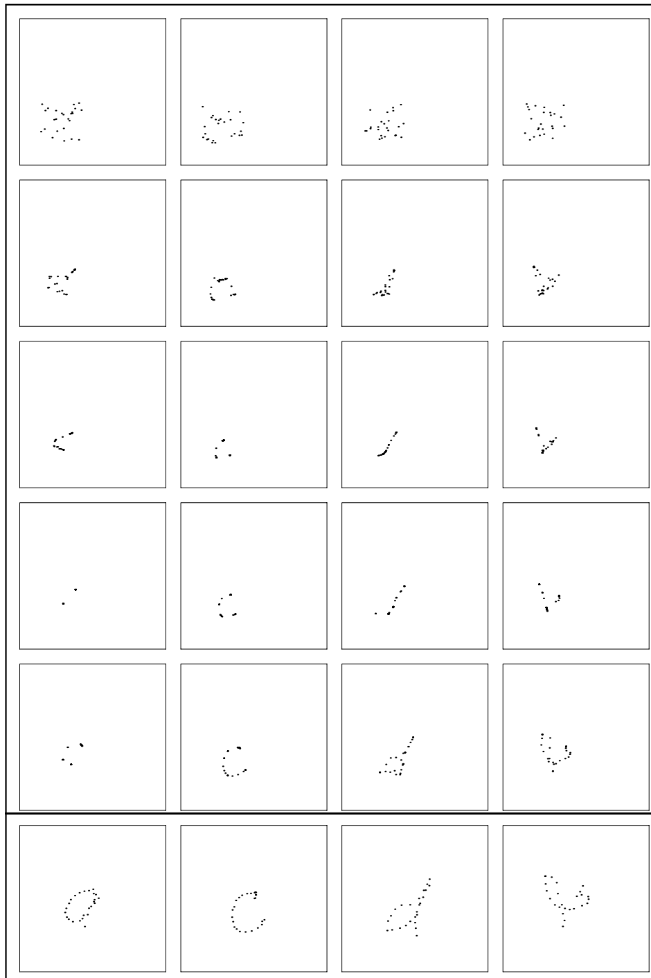
Figure 2: Row (1): initial cluster centers (randomly generated). Rows (2-6): character prototypes (cluster centers) after 4, 16, 64, 128 and 256 iterations.
