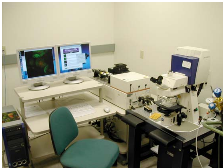
Figure 1. Confocal laser scanning microscope setup dedicated to plant developmental imaging in the Meyerowitz laboratory at Caltech, immediately after installation (photo taken 4/26/04). This is a centerpiece and a major investment of the FIBR Computable Plant project and is now producing useful imagery.
